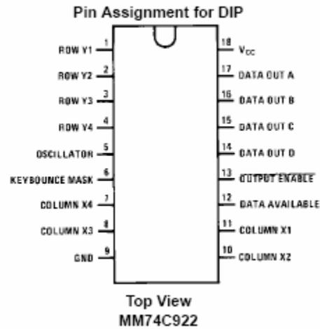
Fig. 4. MM74C92 Pin Assignment
