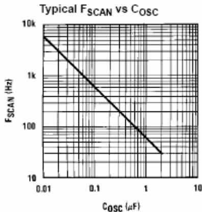
Fig. 2. Keypad scan rate capacitor
