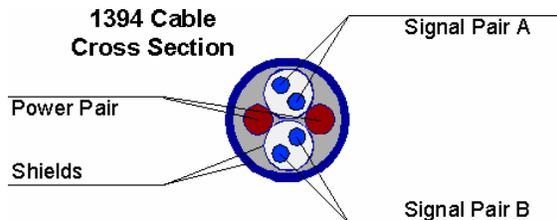
Cable power ranges from 8 to 40 Vdc at 1.5 amps. It is used to power devices and maintains physical layer continuity when a device is powered down or malfunctioned.
