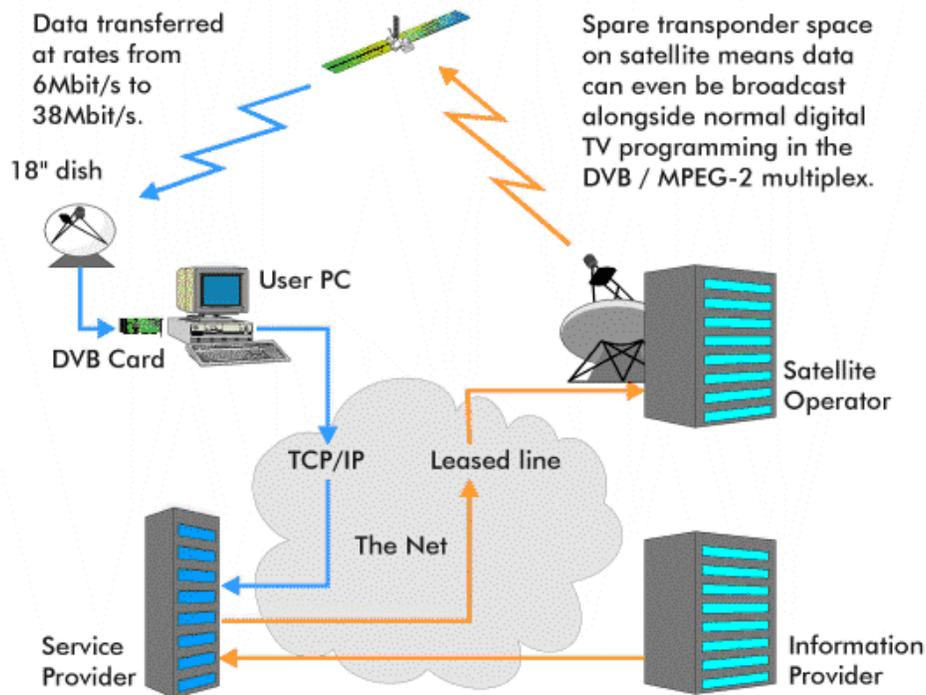
For standard 6, 7 or 8 MHz TV channels, the DVB standard offers a data throughput potential of 6 - 38 Mbps.
