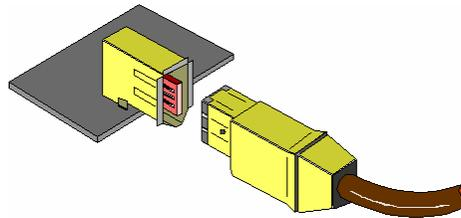
The robust connector is derived from the Nintendo GameBoy. It is small and easy to blindly insert. There are no terminators, or manual IDs to be set.
