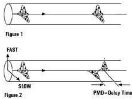
Single-mode fibers support two quadrature polarizations. Perfect fibers would propagate both components at exactly the same velocity. However, in practice, the two components may travel at different velocity and arrive at the end of the fiber at different times.
