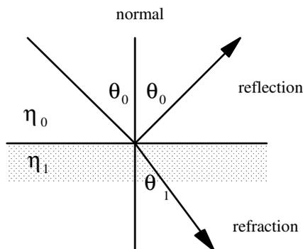
By convention, the angles involved in reflection and refraction are measured with respect to the normal at the point of contact. All three components are in the same plane [there are some exceptions]. In the above illustration, the plane of incidence is the paper.
