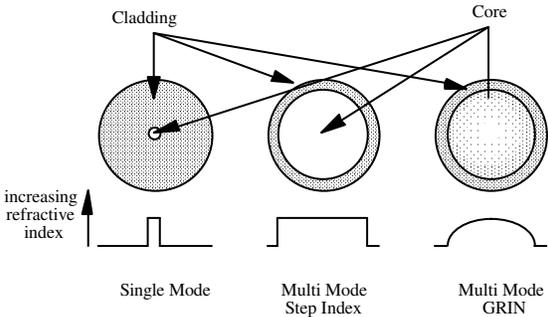
Single mode fibers have a core diameter of 8-10  $\mu\text{m}$ .
