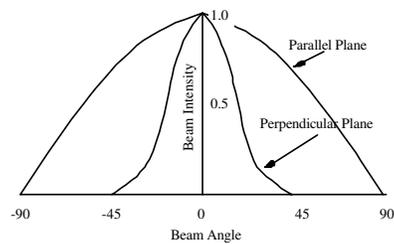
LEDs can be fabricated as surface or edge emitting devices. LDs on the other hand, are currently fabricated only as edge emitters. Edge emitters tend to concentrate the energy and have higher coupling efficiencies than surface radiators.
