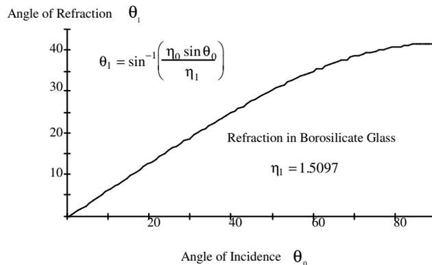
Snell's law has its limitations. At a high angle of incidence, normally transparent objects become excellent reflectors. It also does not take into account the polarization or wavelength of light. The relationship between angle of incidence, amount of reflection, and degree of polarization, is quite complex.
