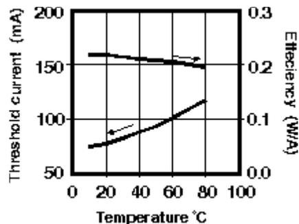
Laser efficiencies are typically about 0.3 mW/mA at 25° C, and drop about 0.01 mW/mA for 10°C increase in temperature.
