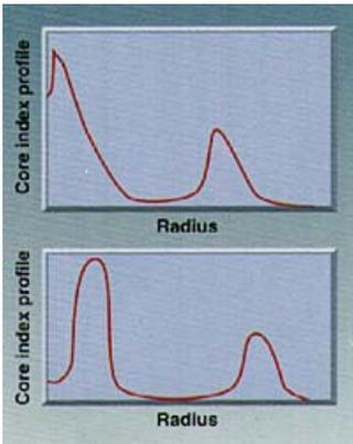
Large-effective-area fiber designs under development include profiles with a triangular central region and outer ring (top) and dual-ring design (bottom).
