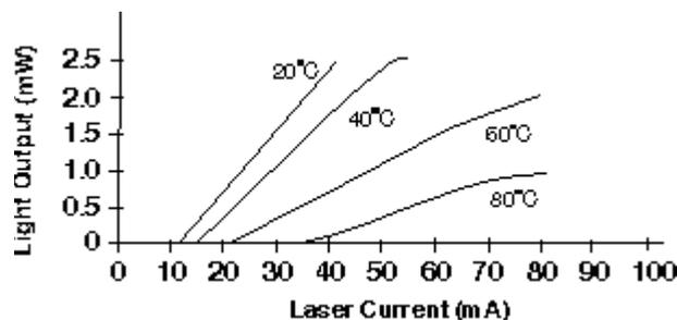
It plots the drive current vs. the output light intensity. It is used to determine the laser's operating point and threshold current. The laser threshold typically increases and the efficiency decreases with temperature.
