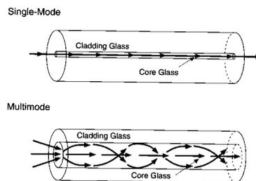
It might appear that multimode fibers have higher information carrying capacity, because they have a larger core and can therefore pass more light. However, the opposite is true. Single mode fibers support higher data rates.
