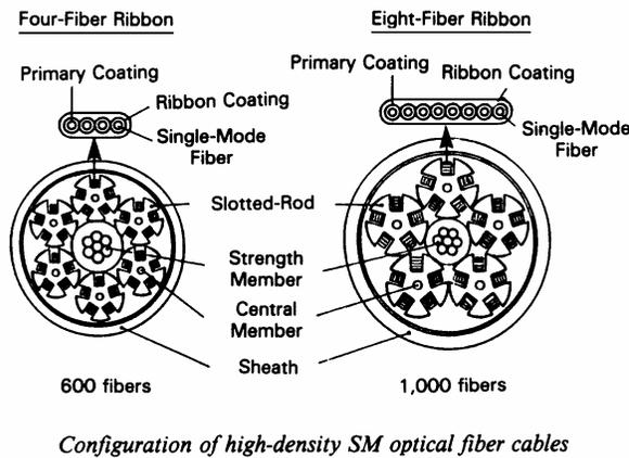
Configuration of high-density SM optical fiber cables
