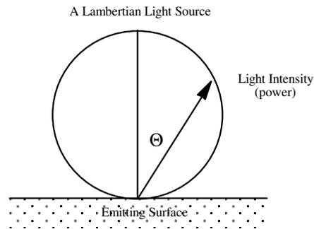
The beam intensity on a surface radiator is symmetric about the radiation axis. However, this is not the case with an edge radiator.
