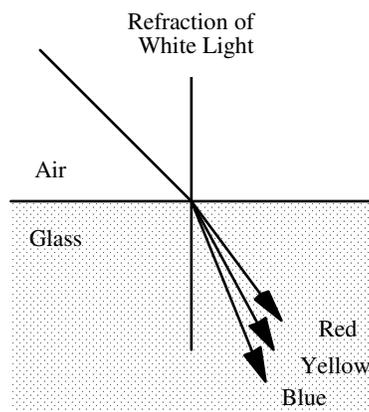
The relationship between the incident and refracted angles is given by Snell's Law:
