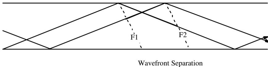
If the waves are in phase at front F1, then they will be out of phase at front F2, since the two rays traveled a different length. The phase relationship on successive reflections remains fixed if the two rays are of the same wavelength.
