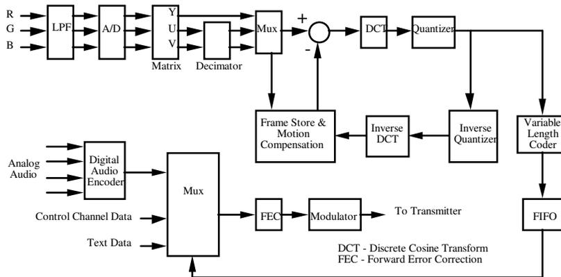
The DCT output is then applied to two separate signal-processing paths. One of these is the variable length coder, which uses an entropy coding algorithm such as Huffman coding, to reduce the number of bits to be ultimately transmitted. The following FIFO transforms this variable speed data into a constant rate.
