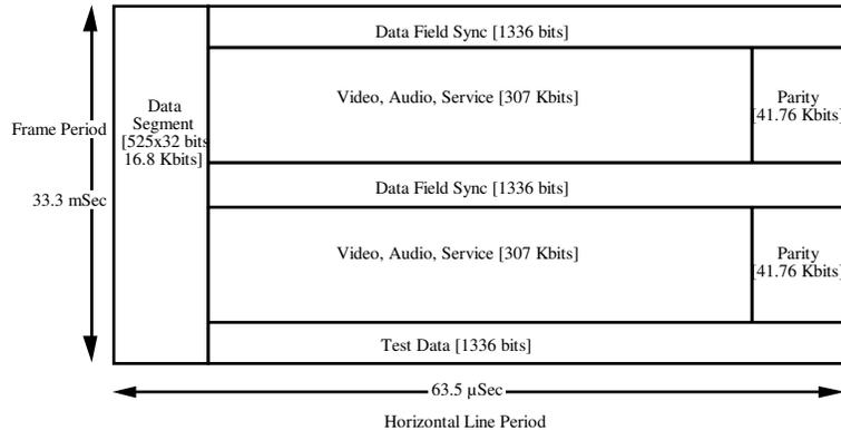
The above format has the additional advantage that because the timing requirements are identical to standard NTSC, there does not have to be any head changes in the HDTV VCR. This means that a digital recorder will be able to both record and playback standard and NTSC and HDTV formats. No need to throw away those old tapes or have two VCRs!
