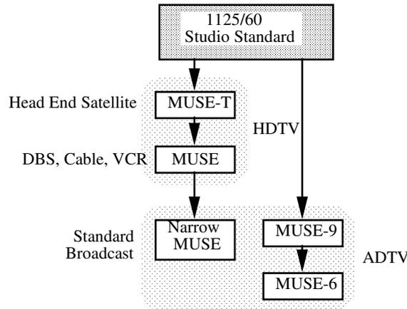
MUSE-E is the highest-level signal in the MUSE family, and has been successfully broadcast over satellite and fiber optic links for several years. This is a complex scheme employing motion-compensated sub-sampling and chroma time compression. Some of the features of this system include:
