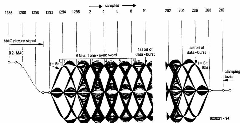
The D2-MAC data burst contains one of two 6 bit line synchronization words [001011 or 110100]. The data burst in line 625, which occurs at the end of a frame, is used to identify even and odd frames. On this line, the synchronization bits are followed by the hexadecimal pattern 55. This is followed by the hexadecimal pattern 65AEF3153F41C246 preceding even number frames, and its inverted form preceding odd numbered frames.
