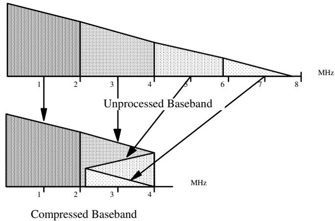
Since the standard TV receiver would display 345 lines, approximately 160 lines are left blank or masked. MUSE-6 uses the masked lines to cram in all of the additional video information that is needed by an ADTV receiver to display a 690-line image. The high frequency components associated with this additional information are folded over to fit into a standard NTSC channel.
