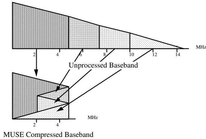
The baseband signal contains 1125 scanning lines. This is reduced to 750 prior to broadcasting by the MUSE process. Field and frame-offset sub-sampling are used on stationary parts of the picture, but only line-offset sub-sampling is used on moving portions. The receiver uses interpolation to reproduce the original image.
