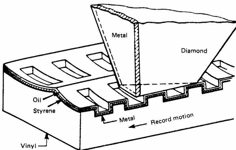
Capacitive stylus and Inconel-coated disc. (RCA Corp.)
