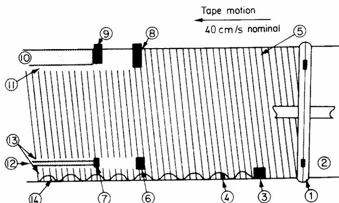
Quadruplex videotape recorder-arrangement of tracks, 1 head-drum, 2 tape, 3 control track head, 4 edit pulse, 5 video tracks 0.25 mm wide with 15.9 mm guard band, 6 cue track erase head, 7 cue track record/reproduce head, 8 audio trace erase head, 9 audio track record/replay head, 10 audio track, 1.78 mm wide, 11 guard band, 0.5 mm wide, 12 cue track 0.5 mm wide, 13 cue track bands 0.25 mm wide, 14 control track 1.27 mm wide
