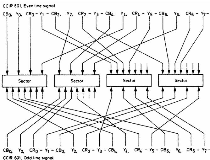
A 50 line segment is split into four sectors and the video data is distributed between the sectors according to a pre-arranged program. The terms  $Y_0$  (luminance),  $CB_0$  (colour components) are time coincident. Where a '-' occurs it indicates there is a separation in time between the components
