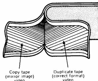
The master and slave tapes can be brought into contact by winding them onto the same take-up spool [bifilar winding], or they can be wound on separate spools and momentarily brought into contact [dynamic winding]. With the dynamic method, as many as six duplicates can be simultaneously made. It takes six minutes to duplicate a one hour program with this method.
