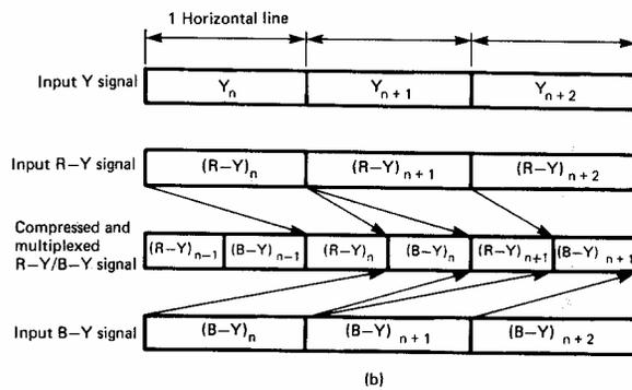
*Betacam chrominance processing. R-Y and B-Y signals are compressed into time of a single line. (a) waveform of compressed signals; (b) time compression and multiplexing system; (c) block diagram of the video signal system (page 166)*
