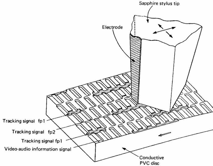
VHD conductive disc and stylus. (Victor Company of Japan, Ltd.)
