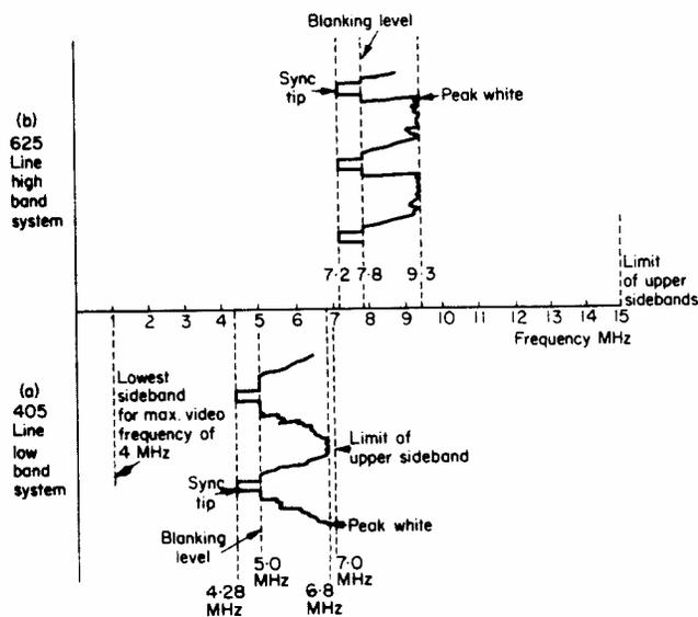
Unlike standard FM, the carrier is deviated in only one direction since the baseband signal is DC. The FM carrier is effectively clamped to the sync tip of the composite video signal. It is also interesting to note that the FM carrier frequency is only slightly higher than twice the highest frequency in the baseband signal.
