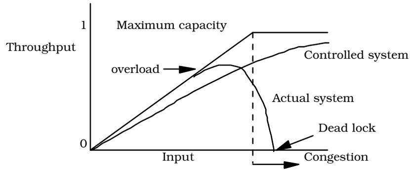
Traffic control governs the number of packets entering and using the network, and can be broken into two components, flow and congestion
