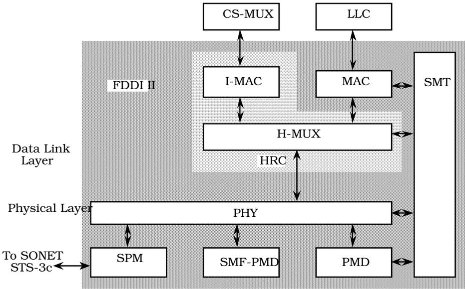
FDDI II adds circuit switch capabilities to the packet switch nature of basic FDDI. It does this by adding a hybrid ring control [HRC] between the MAC and physical layers. The HRC is able to partition the 100 Mbps data stream into multiple streams, capable of handling packet or isochronous data. The
