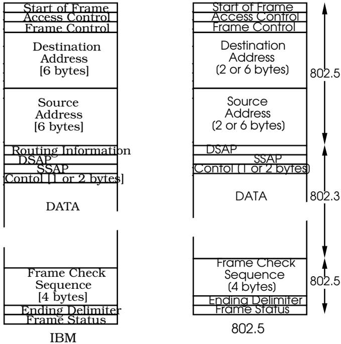
The token ring uses active taps. As a result, only the next station in the ring actually sees the token when it is broadcast. If a station is not going to transmit any data, it regenerates the token on its output port. If the station transmits data, that data will continue to circulate around the ring until it is removed by the originator.
