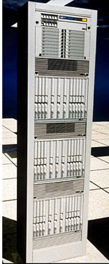
The Magellan Concord system can segregate, prioritize, and manage different types of traffic. 128 QO classes are supported
