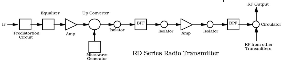
The IF input to the transmitter is a 70 MHz, 64 QAM signal. Since the output amplifier compresses high amplitude signals, a pre-distortion circuit applies emphasis to the high amplitude IF components, thus allowing the output amplifier to operate at its maximum power. This has the overall effect of improving the systems linearity, and help lower the bit error rate to  $10^{-13}$ .
