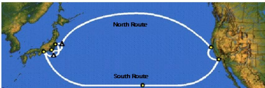
The Japan-U.S. Cable Network has 3 landing points in the United States and 3 in Japan with approximately 21,000km of 8 (4 pairs) fiber submarine cable in a self-healing ring. It will initially operate at 80 Gbps (512 STM-1s) and later at 640 Gbps (4,096 STM-1s).
