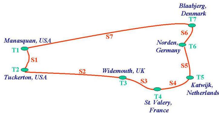
It will span 15,000 km using WDM and SDH technology. The TAT-14 cable will have a total transmission capacity of 640Gbps.
