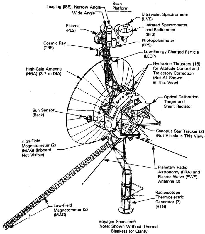
Fig. 2. Voyager spacecraft. The subsystems are shown by callout. The 3.66 m diameter antenna is a highly visible feature.
