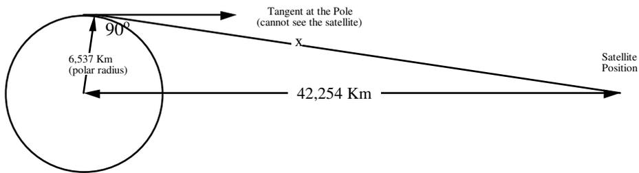
The transmission path length can be found by applying Pythagorean Theorem:
