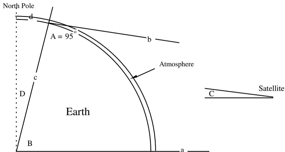
By applying the law of sines, a better approximation of the maximum path length can be determined, as well as the minimum distance from the pole required to see the satellite.
