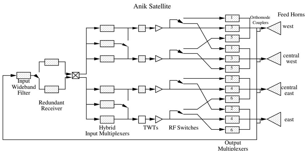
The uplink signal from all antennas are coupled from the horn antennas to the receiver section by orthomode couplers. These respond only to the vertically polarized signal. The received signal is then amplified and down converted to the downlink frequency band.
